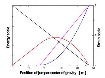
a) Let the zero of the coordinate system be located at the initial position of jumper gravity centre (56 m above the ground level) and jump length is measured from this point downwards the ground along the horizontal axis. In the above sketch there is a graph of four important physical quantities, calculated for the heaviest jumper from the moment of jump start until the moment of reaching the lowest jump point. These four quantities are:
